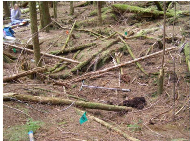
Photo 2. One of the smaller sinkholes examined with test pit exposing thick organic soil in centre, along with soil corer.
