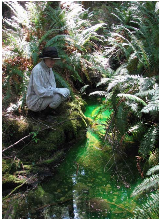
Photo 8. Fluorescein dye appearing at Corner Spring one week after dye injection.
